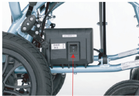
Main power switch (Manual mode switch)
